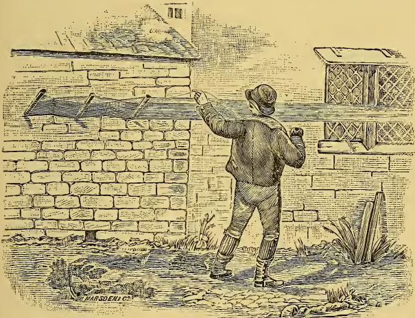
FIG. 150.—PEG WARPING, AN ANCIENT ENGLISH METHOD.
